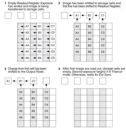
Figure 49. Non-Overlapped Mode Exposure and Readout
